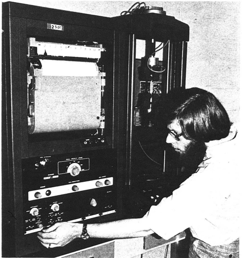
John Mentch, a paper science student, runs stress tests on some paper products. Photo by Roger Barr.
