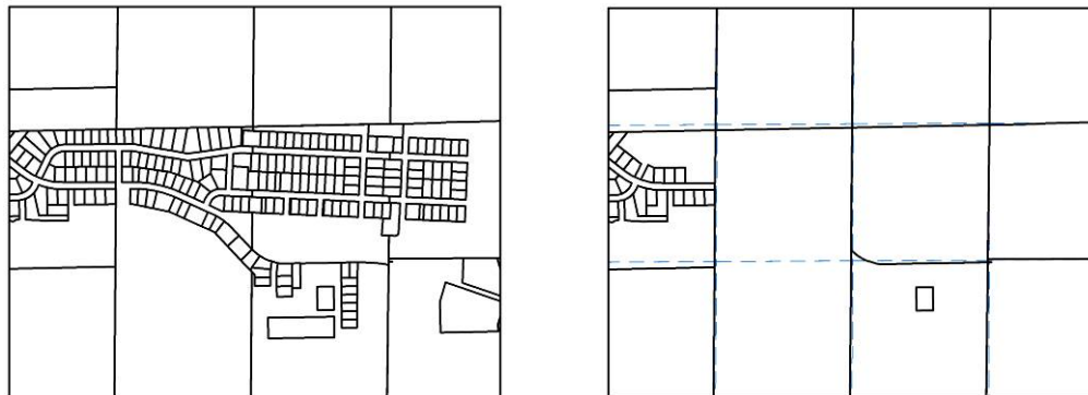
Figure 13. Snapping to section lines (blue hashes), parcels were cut to create tax parcels that did not exist in the digital tax layer.
