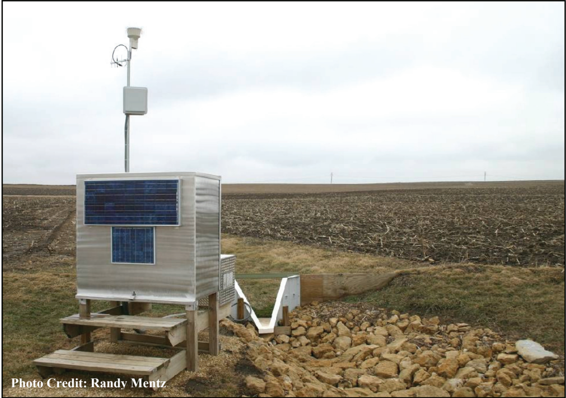
Figure 5 - USGS Edge-of-Field Monitoring Station and Flume Design
