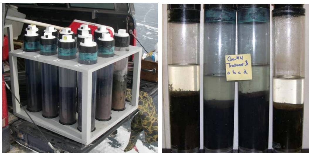
Figure 4. Sediment cores taken in Shawano Lake
